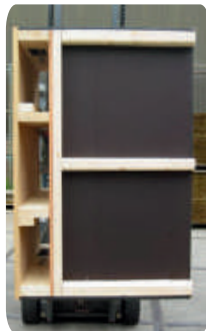
With extra provision, the pallet can be turned over easily by a forklift.
