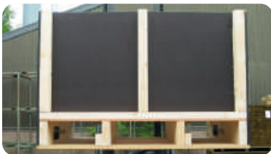
With extra provision, the pallet can be turned over easily by a forklift.
