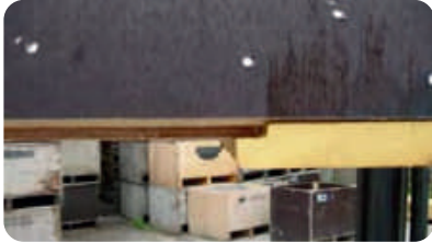
Pallet bottom closed by 9mm plywood.
