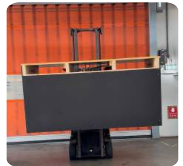
Box cannot move between the pile. The pallet cannot be damaged. This enables a smooth dosing of the product.
