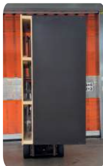
With extra provision, the pallet can be turned over easily by a forklift.
